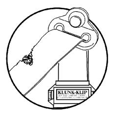
Check to make sure that the D-loop web guide is rotating properly. If the guide is not rotating properly, the webbing will pull at the wrong angle through the guide, accelerating wear.
