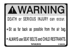
Any queries concerning the SRS system should be directed to an authorized Volvo Truck dealer. There is no maintenance required for the SRS system until the date on the warning label located on the left hand sunvisor.
