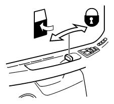
Press button 2 to lock both doors or unlock the passenger door. (Optional)
