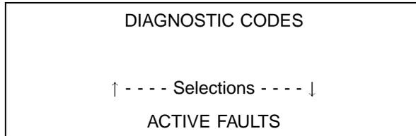
**Note:** As with all menu options, use the up or down arrow to scroll to the desired function, and press ENTER to begin the function. To end use of a function, press the FUNCTION key. This will return you to the previous screen (refer to the Pro-Link/MPC operator's manual for more detailed information about these functions).
