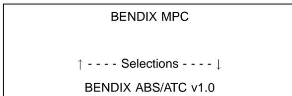
With BENDIX ABS/ATC v1.0 on the bottom line of the display, press ENTER to continue to the "Bendix ABS/ATC Application Menu Structure."
