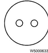
2-pin sensor connector (not polarity sensitive)
