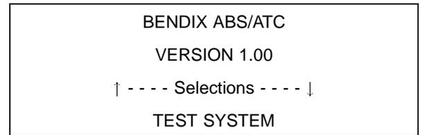
To select the "Test System" option, press ENTER. This function lets you test the operation of components of the ABS/ATC system. These include:
