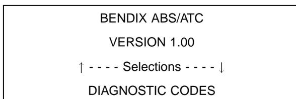
Use the up or down arrows to scroll to the desired option. With the "Diagnostic Codes" option on the bottom line of the display, press ENTER to continue.
