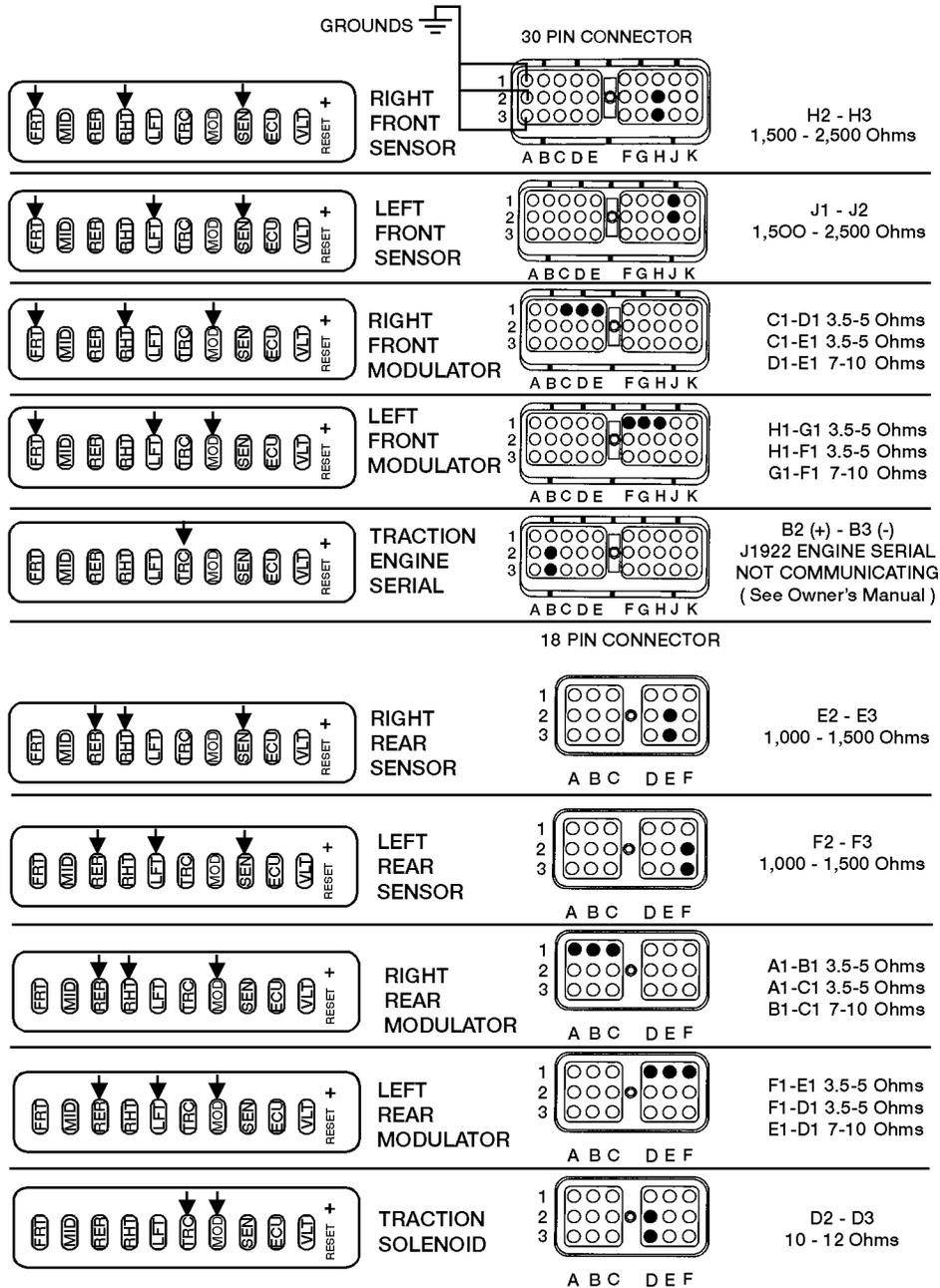
ALL CONTACTS ABOVE SHOULD NOT HAVE ANY CONTINUITY TO GROUND, PIN A1, A2, A3, OR J3 OF 30 PIN CONNECTOR
