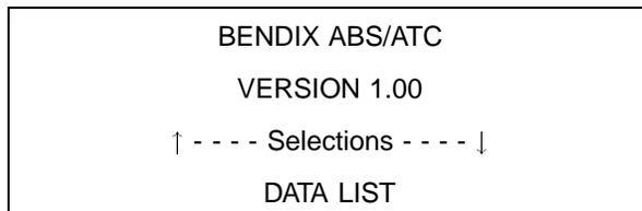
To select the "Data List" option, press ENTER. This lets you view data list parameters in sequence of operation. Press FUNCTION to exit back to the main option menu.
