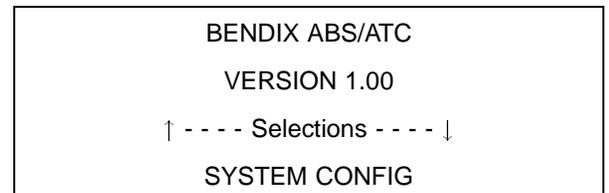
To select the "System Configuration" option, press ENTER. This function lets you view and edit the configuration of the ABS ECU system. This includes:
