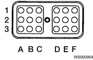
18-pin Metri-pack connector (on ECU)
