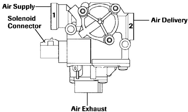
Connect the air supply line to port 1 of the valve. Connect the delivery line to port 2.
