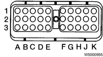
30-pin Metri-pack connector (on ECU)
