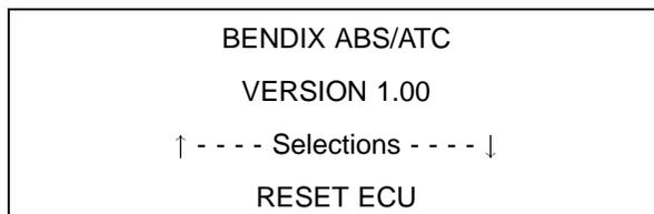
To select the "Reset ECU" option, press ENTER. This function lets you reset the ABS ECU. Press FUNCTION to exit back to the main option menu.
