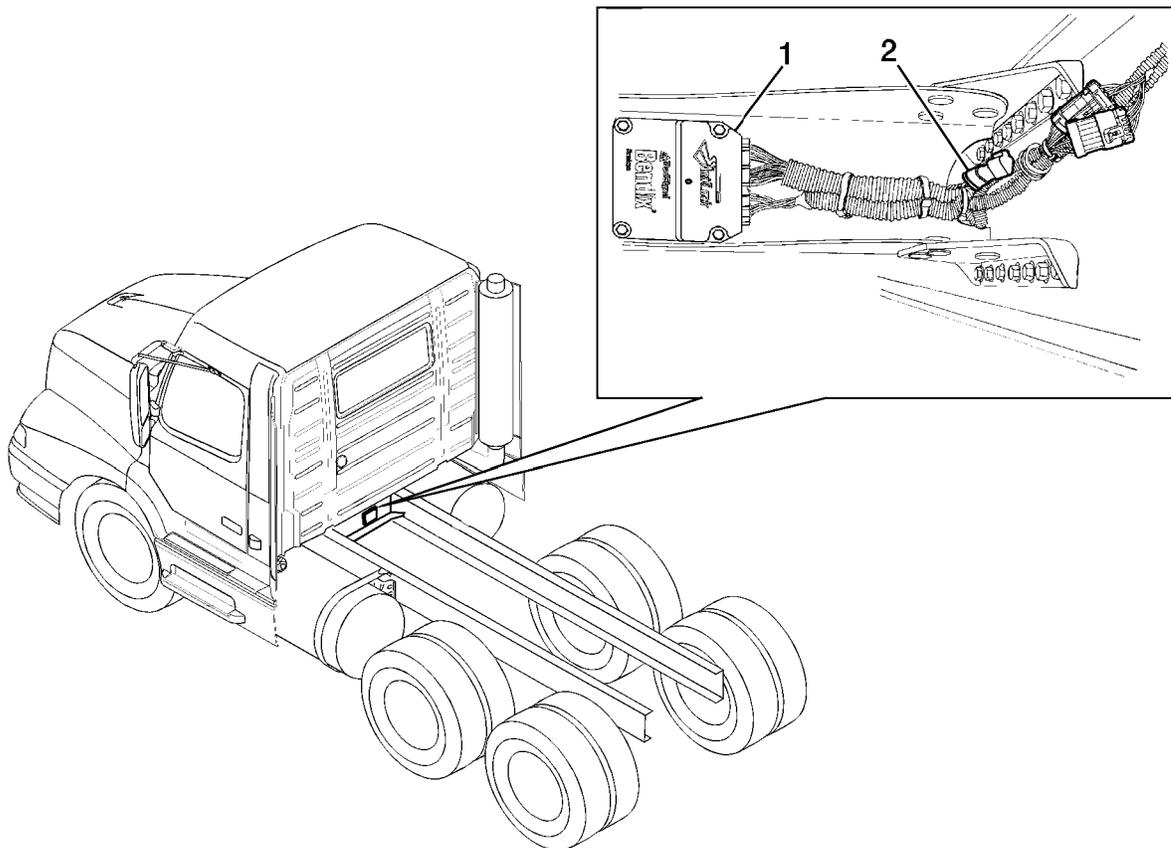
ECU location: rear side of crossmember under or near the back of the cab.
