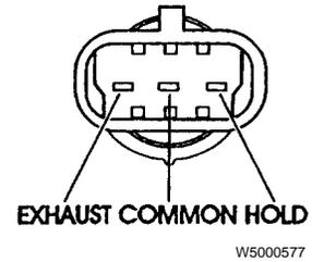
3-pin Packard modulator valve connector
