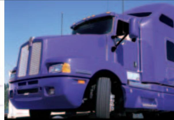
State-of-the-art steering geometry delivers up to 54 degrees of wheel cut – producing a curb-to-curb turning circle of just 56 feet on a model with 165-inch wheelbase.
