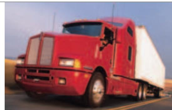
Notice the aerodynamically-sloped hood with its small, contemporary grille. The swept-back fenders. The rounder, smoother, more contoured profile, with an upturned sweep at the top to direct wind upward and over an optimally-curved windshield. There’s a lot less air resistance at the leading edge of this truck. Add full-length chassis fairings, and side extenders and you’ve reduced aerodynamic drag even more.
