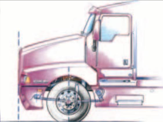
The T600's 46-inch setback front axle helps drivers optimize and maneuver loads with ease.
