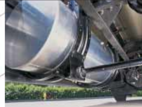
Kenworth fuel tanks are cradled – not hung – supported by durable, high strength brackets made to endure and save you a load of trouble.
